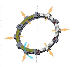
RPM Increases > Wedges Slide Out > EXP Disk Expands > Clutch Engages
